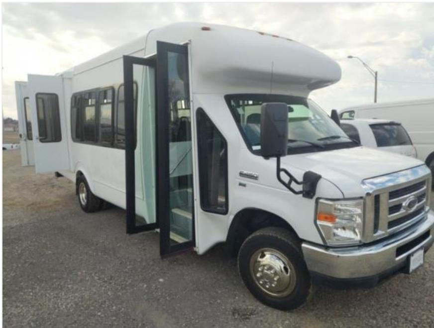
Figure 6 - Ford Econoline E-450 Cutaway Bus outfitted with wheelchair lift<sup>11</sup>
