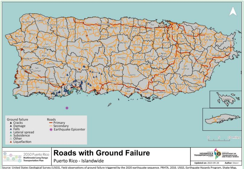
Figure 6.7: Principal Ground Failure Affectations due to 2020 Earthquakes and Puerto Rico Road Network (Primary and Secondary Roads)
