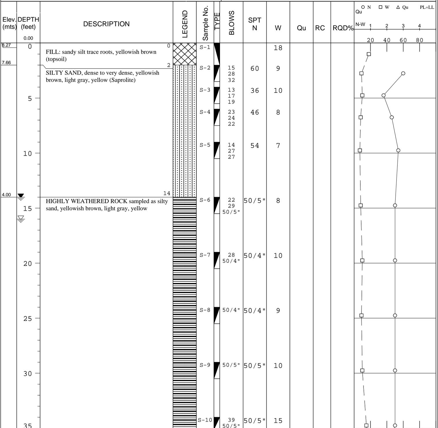
"N" - Number of blows required to drive the sampling spoon a distance of 12 in. with a 140 lbs hammer falling 30 in.
