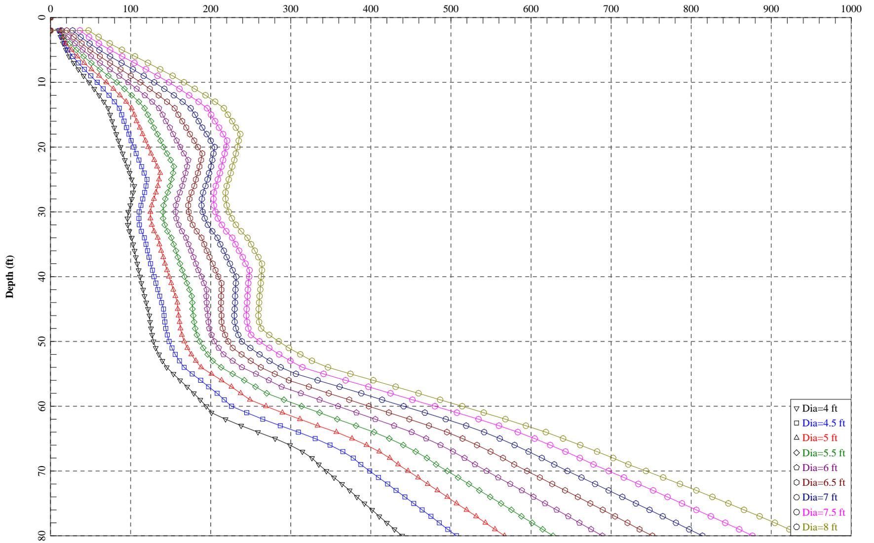
Depth vs. Allowable Compressive Axial Load - Drilled Shaft in Boring no. 5
